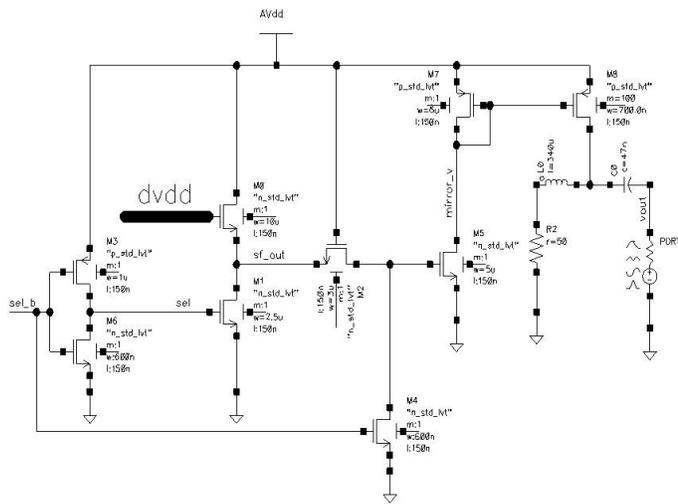
**Figure 5:** Source follower sense amplifier circuit used to detect noise on the digital power rail.
