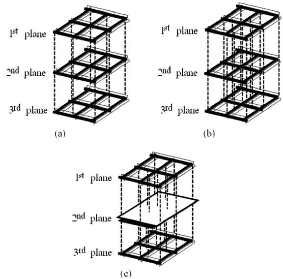
**Figure 1:** Power distribution network topologies. (a) interdigitated power network on all planes with the 3-D vias distributing current on the periphery, (b) interdigitated power network on all planes with the 3-D vias distributing current on the periphery and through the middle of the circuit, and (c) interdigitated power network on planes 1 and 2 and power/ground planes on plane 2 with the 3-D vias distributing current on the periphery.
