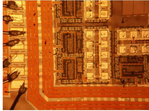
**Figure 6:** One quadrant of the test circuit examining noise on the power distribution network.
