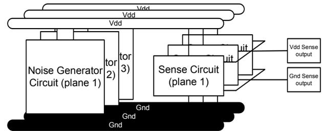
**Figure 2:** Circuit used to analyze power and ground noise.
