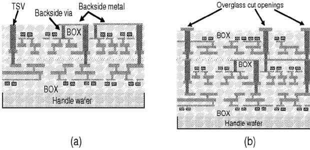
**Figure 3:** Cross-sectional schematic of a 3-D circuit based on the MITTLL process, (a) an intermediate step and (b) fully fabricated 3-D stack [11]. The second plane is flipped and bonded with the first plane, while the third plane is bonded face-to-back with the second plane. The backside metal layer and vias and the through silicon vias are also shown.
