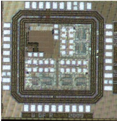
**Figure 4:** Fabricated test circuits examining three different power distribution networks and a distributed DC-to-DC power converter.
