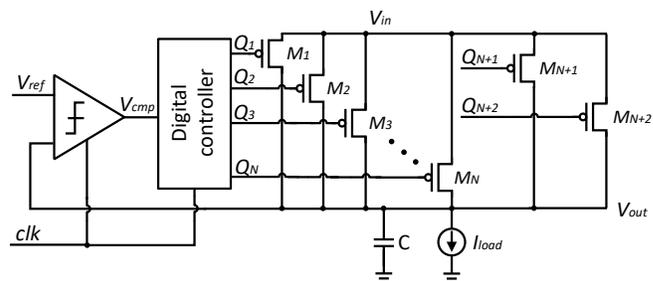
Fig. 1. Schematic of DLDO with LCO mitigation.
