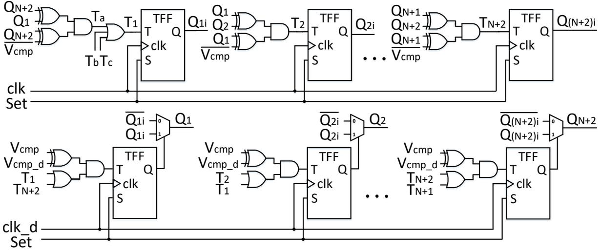
Fig. 3. Proposed  $N + 2$  bit unidirectional controller for reliability enhanced on-chip DLDO with LCO mitigation.
