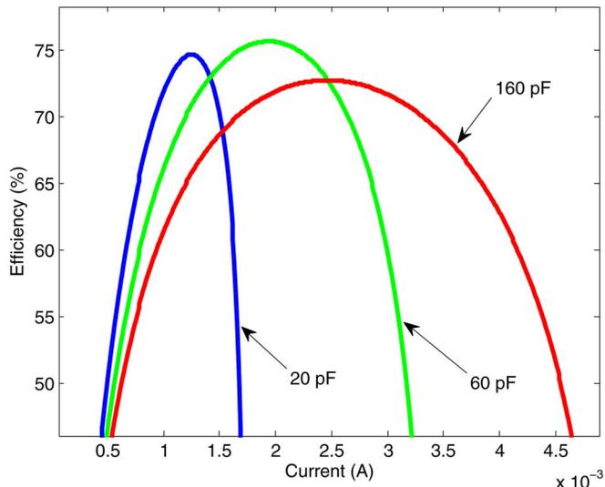
Fig. 5. Power conversion efficiency of various SC voltage converter with different flying capacitor values. A smaller converter provides maximum power efficiency when the load current is lower whereas a larger converter can provide better efficiency under higher output current.
