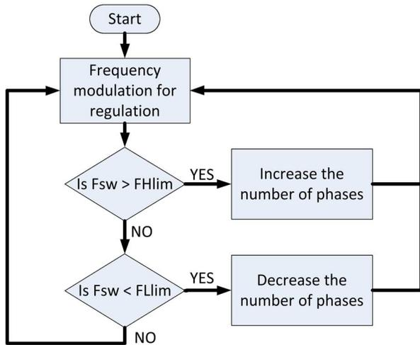
Fig. 7. Proposed converter-gating algorithm that enables workload aware activity management of distributed SC voltage converters.
