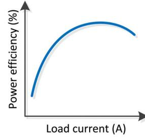
Fig. 3. Power efficiency of buck converters. The efficiency graph exhibits a nonmonotonic behavior and the maximum power efficiency is obtained at a certain output current.
