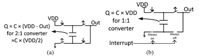
Fig. 8. Amount of charge transferred to the output node in a single cycle for (a) a conventional 2:1 SC voltage converter and (b) a 2:1 converter that is configured as a 1:1 converter by controlling the illustrated switches. 1:1 configuration provides two times more charge to the output node in a given cycle, improving the response time.
