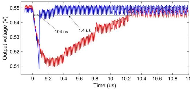
Fig. 10. Transient response of a 2:1 SC converter when the load current increases from 1 mA to 3 mA. The response time for a conventional 2:1 SC voltage converter (shown in red) is 1.4  $\mu$ s. When the proposed adaptively configurable voltage converter, shown in Fig. 8 is used, the response time reduces to 104 ns.
