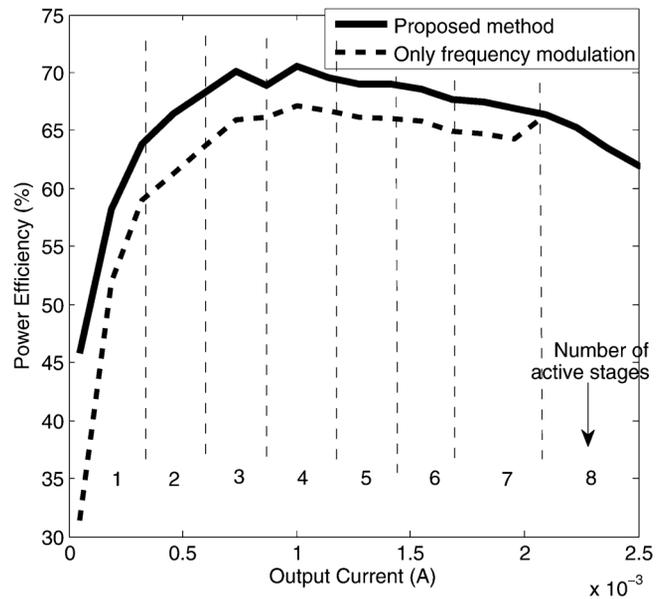
Fig. 9. Power conversion efficiency of an eight stage interleaved SC voltage converter with and without applying the proposed converter-gating technique. The power conversion efficiency is increased  $\sim 5\%$  with negligible area overhead by utilizing the proposed technique.
