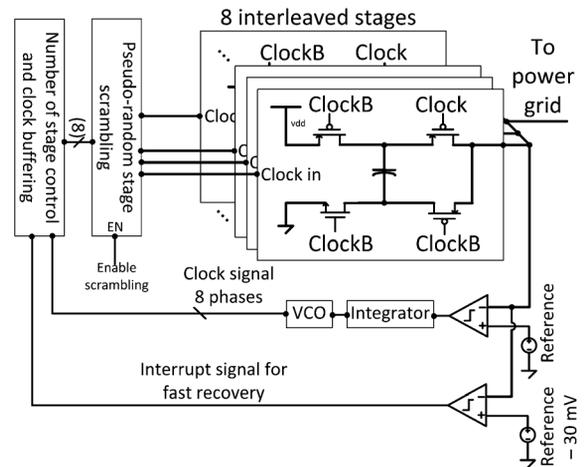
Fig. 6. Top level schematic of the proposed converter-gating system.
