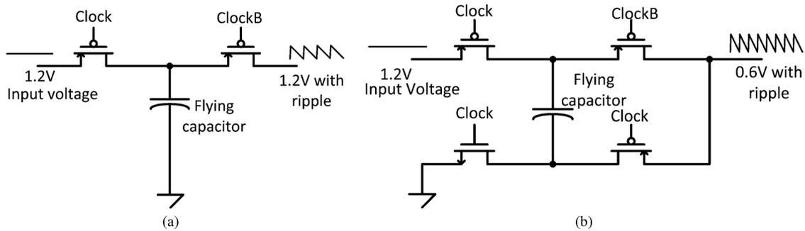
Fig. 4. Two different topologies for SC voltage converters where the MOSFET switches are controlled with nonoverlapping *Clock* and complimentary *ClockB* signals. (a) 1:1 converter with two switches and a flying capacitor. (b) 2:1 converter with four switches and a flying capacitor.
