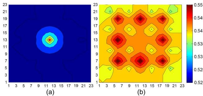
Fig. 11. Voltage map of the power grid when the load circuits are uniformly distributed. (a) All of the eight stages of an SC voltage converter are connected to the center of the power grid. (b) All of the eight stages of an SC converter are distributed uniformly.
