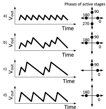
Fig. 13. Output voltage ripple of a four phase interleaved SC voltage converter with different number of active stages. (a) All stages are active. (b) One stage is deactivated. (c) Two adjacent phases are deactivated. (d) Two symmetric phases are deactivated.
