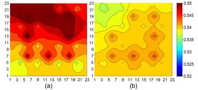
Fig. 12. Voltage map of the power grid when the load circuits located at the upper-left corner of the power grid enters idle state and all of the eight stages of an SC converter are distributed uniformly. (a) All of the converter stages are active. (b) Individual voltage converter stages that are close to the idle circuit block are deactivated with the proposed converter-gating technique.
