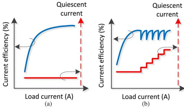
Fig. 1. Current efficiency of different LDO regulators. (a) Current efficiency of an LDO regulator increases monotonically with the load current when the quiescent current is constant. (b) Adaptively controlling the quiescent current based upon the load current can improve the current efficiency.
