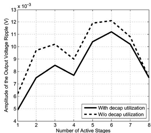
Fig. 14. Amplitude of the output voltage ripple when the inactive converter stages are utilized as decoupling capacitor (solid line) and without decoupling capacitor utilization (dashed line). 20% reduction in the output voltage ripple can be achieved with the proposed decoupling capacitor utilization.
