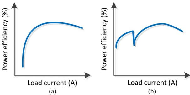
Fig. 2. Power efficiency of different SC converters. (a) The power efficiency of an SC converter is not necessarily monotonic but the maximum efficiency is typically obtained while delivering a certain output current. (b) Different techniques can be used to improve the efficiency at light load currents.
