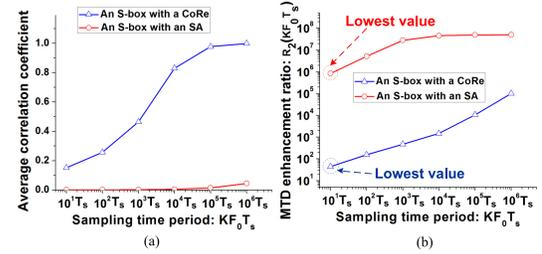
Fig. 5. (a) Average correlation coefficient versus sampling time period  $KF_0T_s$ . (b) MTD enhancement ratio  $R_2(KF_0T_s)$  versus sampling time period  $KF_0T_s$  ( $F_0 = 10$  and  $N = 32$ ).
