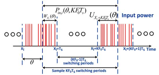
Fig. 4. Input power profile of a cryptographic circuit that employs an SA voltage converter under LPA attacks when the attacker selects a variable number of clock periods as one sample of input power data.  $X_i$  is the starting time point of the first switching period for sampling the  $i$ th input power data.
