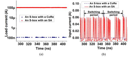
Fig. 6. (a) Load current profile of an S-box that employs a CoRe voltage converter and an S-box that employs an SA voltage converter. (b) Input current profile of an S-box that employs a CoRe voltage converter and an S-box that employs an SA voltage converter.
