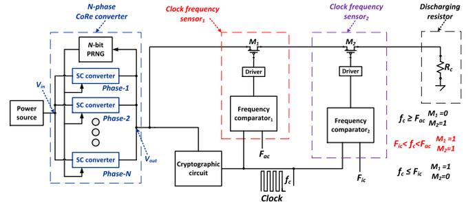
Fig. 1. Architecture of the proposed SA voltage converter.  $N$  is the total number of phases ( $N$  is an even). Switch  $M_{i1} = 1$  ( $i_1 = 1, 2$ ) represents that it is in ON-state and *vice versa*.
