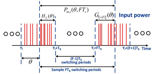
Fig. 2. Input power profile of a cryptographic circuit that employs an SA voltage converter under LPA attacks when the attacker selects a single clock period as one sample of input power data.  $T_s$  is the switching period of the SA voltage converter,  $Y_i$  is the starting time point of the first switching period for sampling the  $i$ th input power data, and  $\theta$  is the phase difference between the switching period and input power data sampling.
