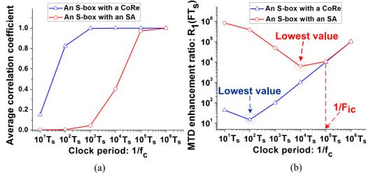
Fig. 3. (a) Average correlation coefficient versus clock period  $1/f_c$ . (b) MTD enhancement ratio  $R_1(FT_s)$  versus clock period  $1/f_c$ .
