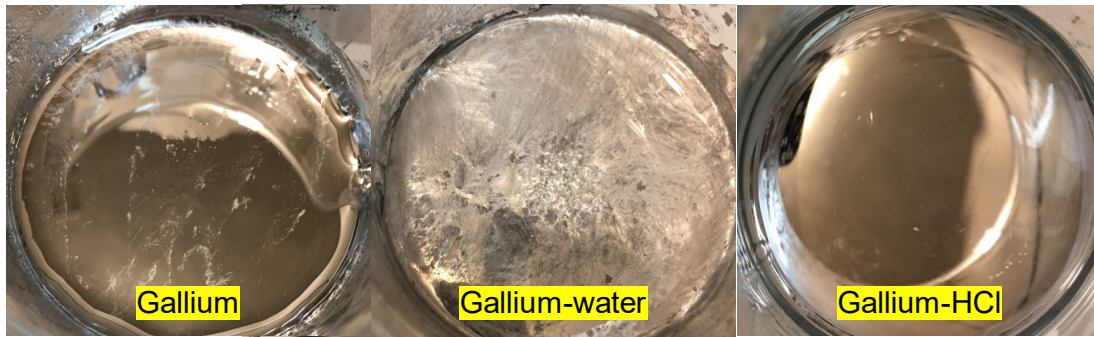
Figure 2.10 Pictures of liquid gallium with different treatments. The treated gallium exhibited significant differences in surface appearance.
