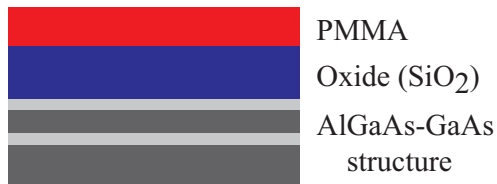
(3) Spin-coat e-beam resist
