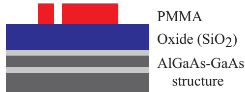
(4) Pattern inverse with e-beam & develop
