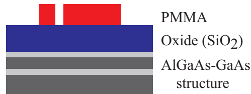
(4) Pattern inverse with e-beam & develop
