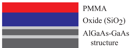
(3) Spin-coat e-beam resist
