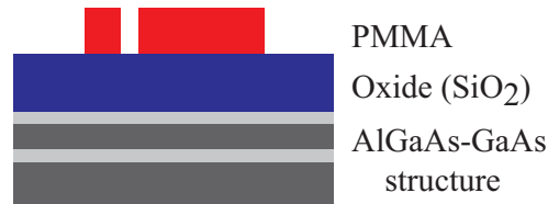
(4) Pattern inverse with e-beam & develop
