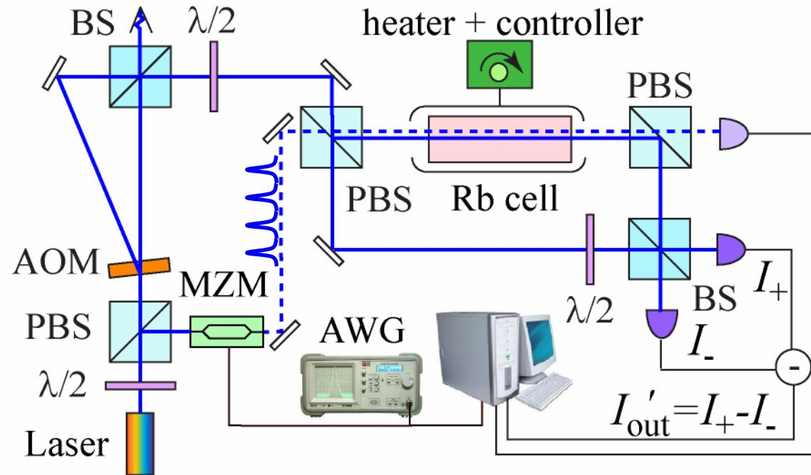
Schematic diagram of the experiment setup of an FT-interferometer using a rubidium cell as the slow-light medium.
