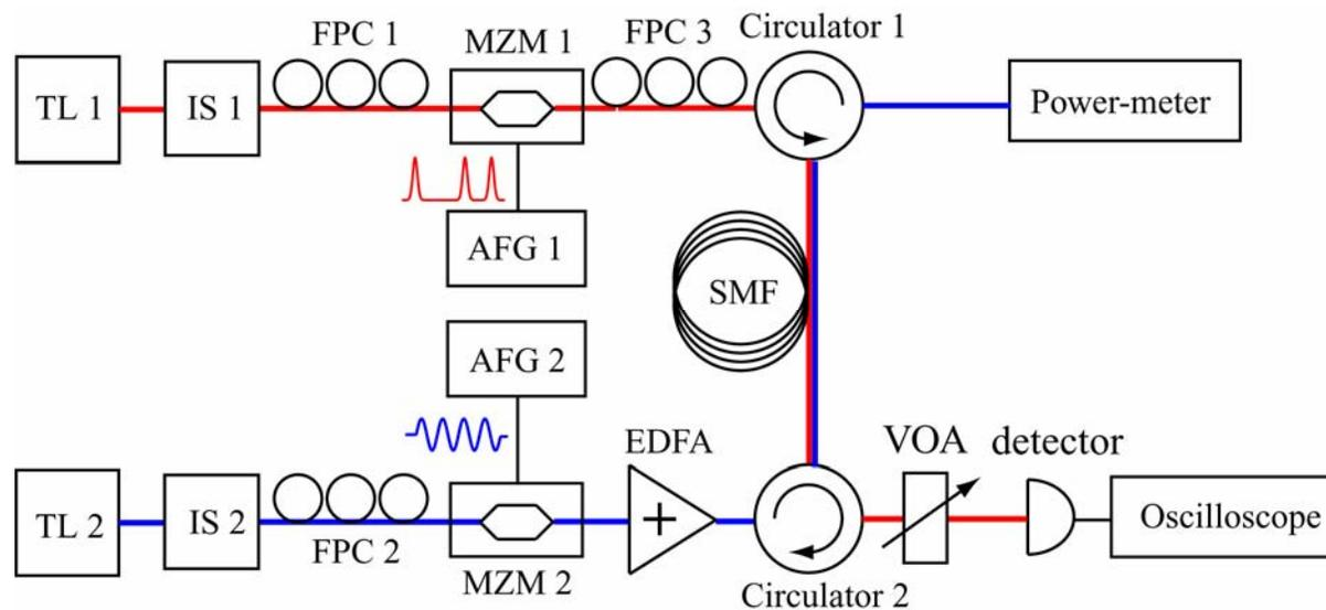
Schematic diagram for the multi-gain-line SBS experiment
