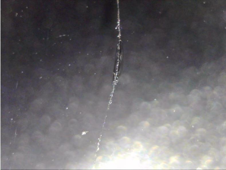
**Picture 5:** Picture of lens under darkfield lighting with source at 60 degrees from the ground. The light from the source can be seen at the bottom of the picture.
