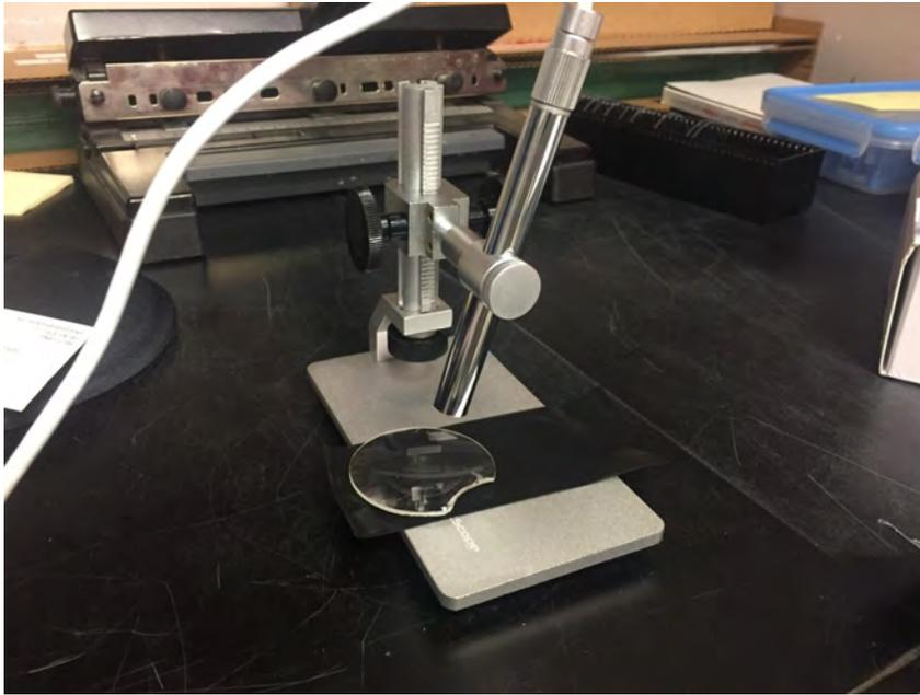
**Figure 1:** Opti-Tekscope imaging a lens surface. The industrial lighting is present and adding ambient light into the system. Black masking tape is used to absorb light from our improvised light source (Not in picture).
