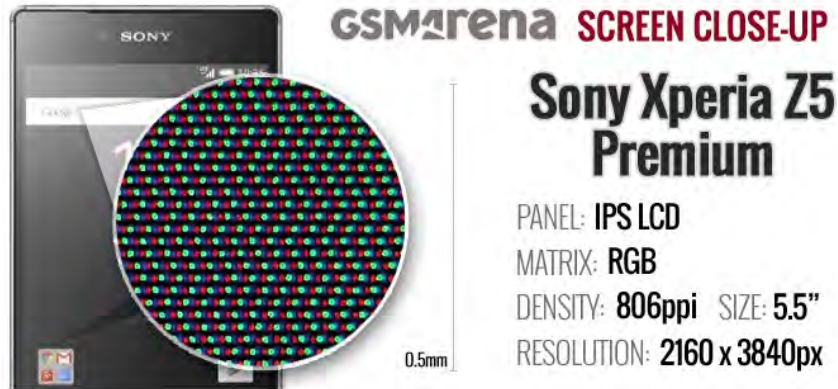
Figure 14. Pixel arrangement of Xperia Z5 Screen. This layout is not an accurate representation of the RGB pixel distribution.
