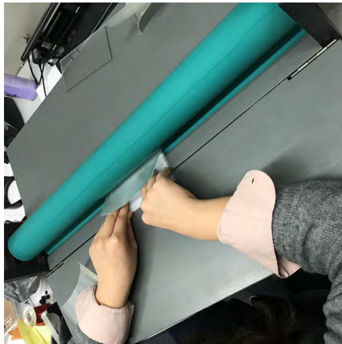
Figure 21. Adhering a lenslet array to an acrylic board using a roller.
