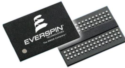
Figure 3.9: An MRAM based main memory from Everspin Technologies [76].
