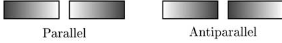
Fig. 2. Current density distribution in the cross section of two closely spaced lines at high frequencies. Darker shades of gray indicate higher current densities. In lines carrying current in the same direction (parallel currents), the current concentration is shifted away from the parallel current. In lines carrying current in opposite directions (antiparallel currents), the current concentrates toward the antiparallel current, minimizing the circuit inductance.
