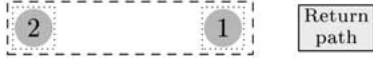
Fig. 5. A cross-sectional view of two parallel current paths (dark gray) sharing the same current return path (light gray). The path closest to the return path, path 1, has a lower inductance than the other path, path 2. The parallel paths can be either two physically distinct lines, as shown by the dotted line, or two different paths within the same line, as shown by the dashed line.
