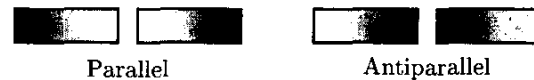
Fig. 2. Current density distribution in the cross section of two closely spaced lines at high frequencies. Darker shades of gray indicate higher current densities. In lines carrying current in the same direction (parallel currents), the current concentration is shifted away from the parallel current, minimizing the circuit inductance. In lines carrying current in opposite directions (antiparallel currents), the current concentrates toward the antiparallel current, also minimizing the circuit inductance.
