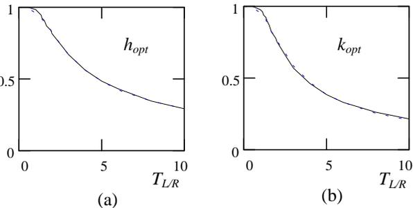
Fig. 4. Numerical solutions of (10) as compared to eqs. (14) and (15). a)  $h_{opt}$  as compared to (14). b)  $k_{opt}$  as compared to (15). Numerical solutions are shown by the solid line while (14) and (15) are shown by the dashed line.
