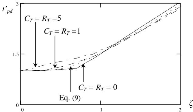
Fig. 2. Comparison of the accuracy of (9) to AS/X [14] simulations of the time scaled 50% propagation delay  $t'_{pd}$  of an  $RLC$  transmission line with a source resistance  $R_{tr}$  and a load capacitance  $C_L$ . The propagation delay is plotted versus  $\zeta$  for different values of  $R_T$  and  $C_T$ .
