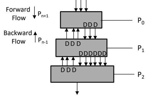
Fig. 4: Forward and backward edges between partitions using the resistive tree current distribution method. The direction of flow determines where the driver is placed since the driver requires four JJs and the receiver requires two JJs. The driver is placed, respectively, at the origin of the forward and backward edges.
