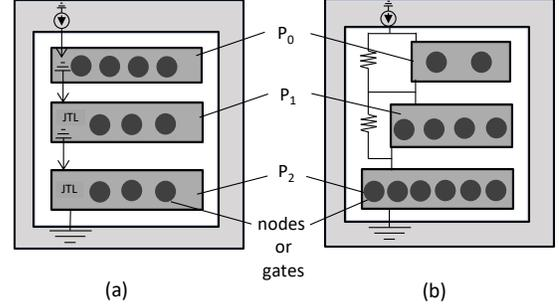
Fig. 2: Serially biased partitioned circuit blocks ( $P_n$ ) on isolated ground planes illustrate the current distribution process, (a) overlap bias current classification with dummy JTLs, and (b) non-overlap bias current classification with a resistive tree
