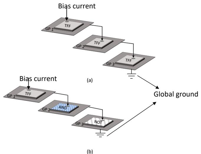
Fig. 1: Serially biased circuits, (a) homogeneous circuits, and (b) heterogeneous circuits
