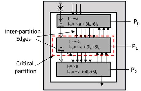
Fig. 3: Inter-partition edges illustrating the critical partitions
