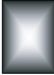
Figure 2.8: Current distribution in the cross section of an interconnect at high frequencies. Darker color indicates higher current density.
