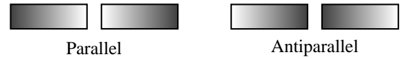
Fig. 2. Current density distribution in the cross section of two closely spaced wires. Darker shades of gray indicate higher current densities. In wires carrying current in the same direction (parallel currents), the current concentration is shifted away from the parallel current, minimizing the circuit inductance. In wires carrying current in opposite directions (antiparallel currents), the current concentrates toward the antiparallel current, also minimizing the circuit inductance.
