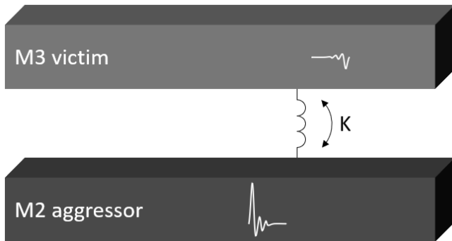
Fig. 9: Inductive coupling between parallel PTLs showing the aggressor and victim lines.
