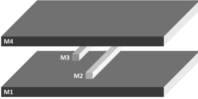
Fig. 4: Two identical parallel PTLs in adjacent layers with signal lines in M2 and M3.
