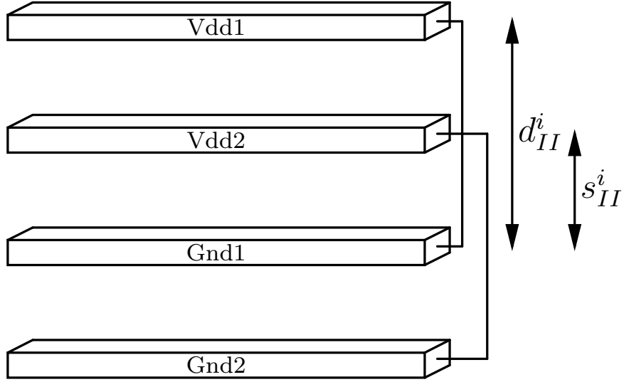
Figure 4.6: Physical structure of a pseudo-interdigitated power distribution grid with DSDG. The distance between the lines making the loops d_{II}^i is two times greater than the separation between the lines.
