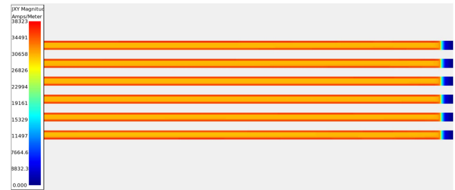
Fig. 3. Current distribution within a stripline with the six parallel line topology.
