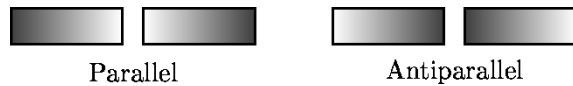
Fig. 2. Current density distribution in the cross section of two closely spaced lines at high frequencies. Darker shades of gray indicate higher current densities. In lines carrying current in the same direction (parallel currents), the current concentration is shifted away from the parallel current, minimizing the effective coupling between the two currents and, therefore, the circuit inductance. In lines carrying current in opposite directions (antiparallel currents), the current concentrates toward the antiparallel current, minimizing the current loop area, and, therefore, minimizing the circuit inductance.
