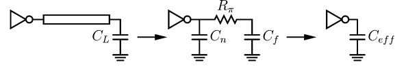
Fig. 3. \pi model representation of a distributed RC interconnect and the effective capacitance.
