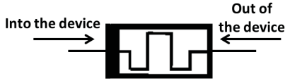
Fig. 1. Memristive device symbol. The thick black line on the left side of the device represents the polarity of the device. If the current flows into the device, the resistance of the device decreases. If the current flows out of the device, the resistance increases.
