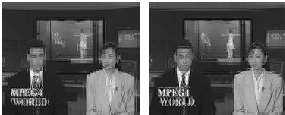
Figure 4: Multiple description coding results: (a) First description only, (b) Second description only
