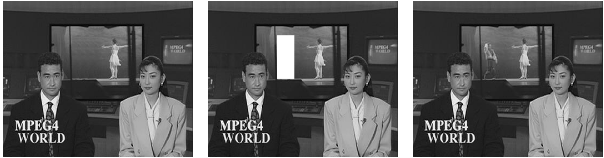
Figure 6: Spatial attack results: (a) Manipulated frame, (b) Detection result, (c) Recovered frame
