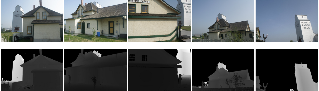
Fig. 6: Sample results for dense depth map estimation. The first row shows five input RGB images captured using a digital camera, and the second row shows the corresponding depth map generated by our method. The corresponding point cloud is shown in the example of Fig. 1.
