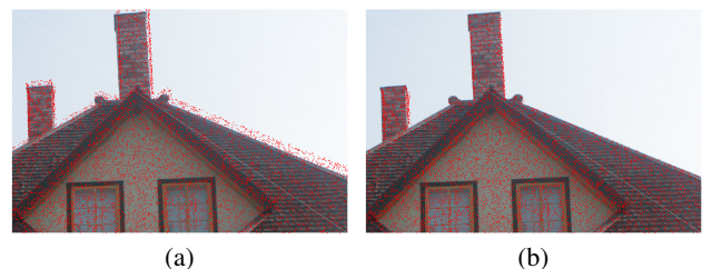
Fig. 7: Sample results for visual comparison of reprojecting points onto image planes between (a) VisualSFM and (b) our method. The image shows the roof region of the building in Meeting Creek . Notice that, in our method, the edge points of roof and chimneys is aligned precisely to the image.
