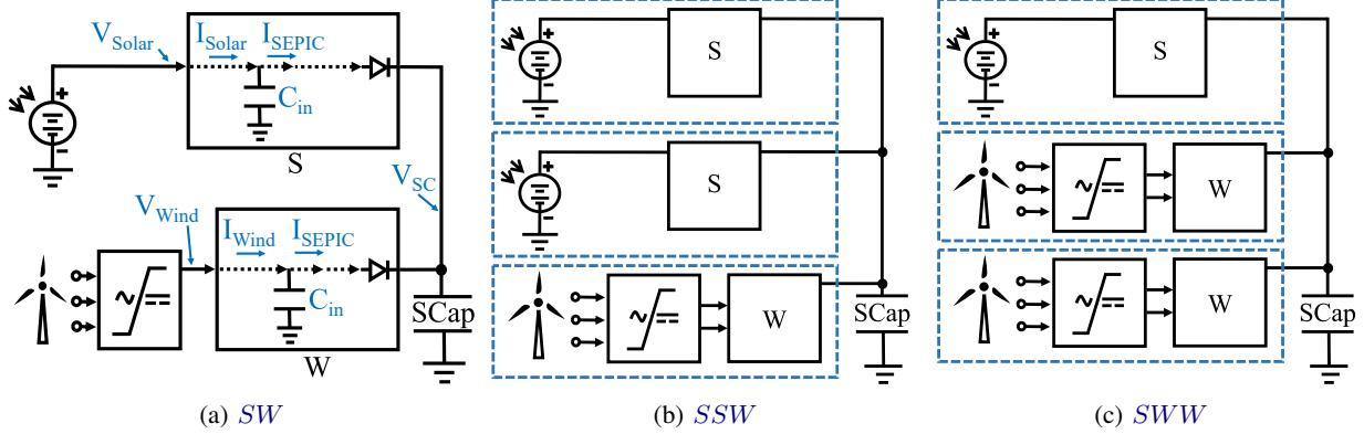
Figure 3: Three example configurations of our proposed hybrid harvesting. The modularity of our architecture allows us to implement a variety of hybrid energy harvesters by incorporating additional solar- and wind-only harvesters.
