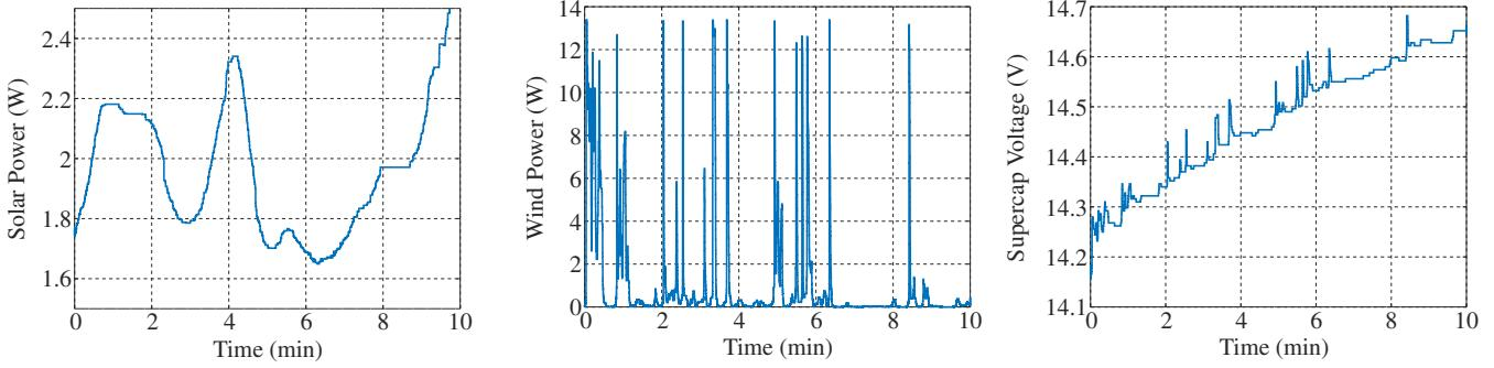
Figure 4: Experimental results for the *SW* harvester. Far left plot shows the output power of solar panel, while the middle plot shows the output power of the wind turbine. The voltage of the supercapacitor energy storage block is depicted in the far right sub-figure. During this period,  $\hat{P}_{\text{solar}} \approx 2 \text{ W}$  and  $\hat{P}_{\text{wind}} \approx 1.7 \text{ W}$  and the average cumulative incoming power is  $\hat{P} \approx 3.7 \text{ W}$ .
