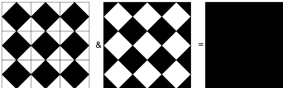
Figure 4. Overlap of out of phase clustered dot halftones at a 50% gray level.
