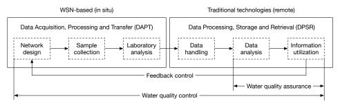
(a) Adaptation of the traditional WQM framework when using a WSN for data acquisition, processing and transfer (DAPT).
