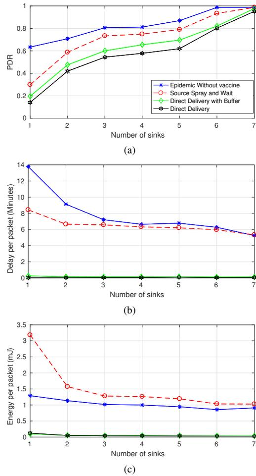
Figure 8: Effect of number of sinks on PDR, average delay and energy consumption per received packet at 4 dBm transmit power for real time tracking.
