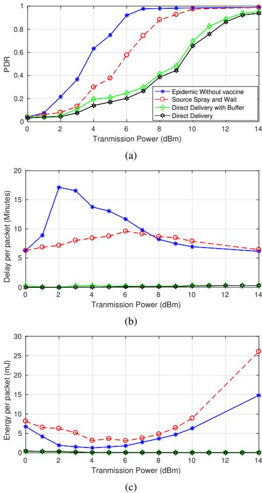
Figure 7: PDR, average delay and energy consumption per received packet for real time tracking in a single sink architecture.
