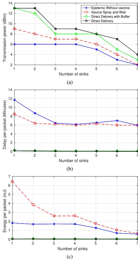
Figure 9: Required transmission power, the corresponding average delay and energy consumption per received packet to achieve 90% PDR for real time tracking in a single sink architecture.
