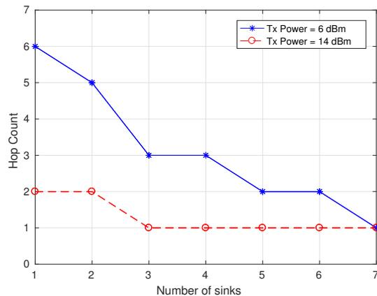
Figure 10: Minimum required hop count in epidemic routing (HopCount) to achieve 90% PDR for real time tracking in a single and multiple sinks architecture.
