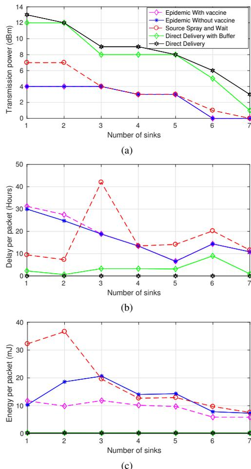
Figure 6: Required transmission power, the corresponding average delay and energy consumption per received packet to achieve 90% PDR for the movement pattern analysis in a single sink architecture.
