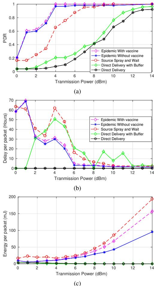
Figure 4: PDR, delay and energy consumption per received packet for the movement patterns analysis in a single sink architecture.
