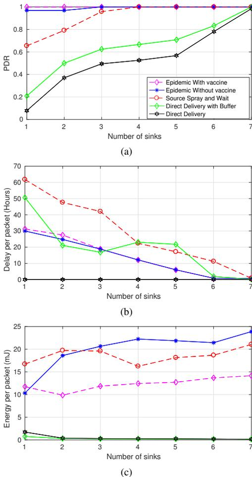
Figure 5: Effect of number of sinks on PDR, average delay and energy consumption per received packet at 4 dBm transmit power for the movement pattern analysis.
