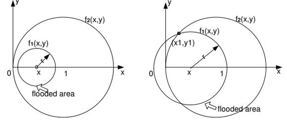
**Figure 2: The intersection area is the region covered by flooding. When  $r < x_0$ , it is  $f_1(x, y)$ ; when  $r \geq x_0$ , it is the intersection of two areas.**
