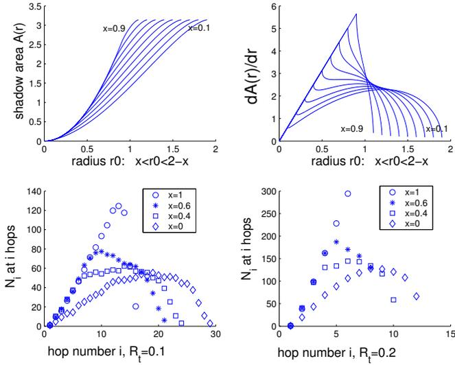
**Figure 3: Area  $A(r)$  of flooded region and the relation between the number of nodes  $N_i$  exactly  $i$  hops away with  $\frac{dA(r)}{dr}$ . Part (1) is the flooded area  $A(r)$ ; part (2) is  $\frac{dA(r)}{dr}$ ; part (3) is the  $N_i$  in a network of 1000 nodes and transmission range 0.1; part (4) is the  $N_i$  in a network of 2000 nodes and transmission range 0.2. Part (3) and part (4) look like a sampling of part (2).**
