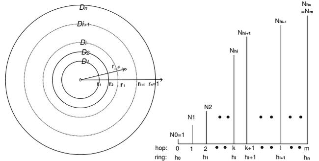
Figure 1: Models of target discovery for large-scale wireless networks. On the left is the geography-based flooding control model, and on the right is the hop-based flooding control model.
