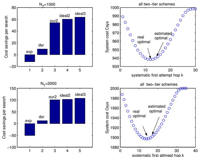
**Figure 6: The cost savings of different schemes for small-scale networks. From left to right labeled as 1 to 5: (1) expansion ring, (2) DSR, (3) our two-tier scheme, (4) the ideal two-tier scheme, (5) the ideal three-tier scheme. The graph on the right shows the system cost for different  $k_{sys}$  of the two-tier scheme. Our estimated points are 13 for 1000 nodes and 16 for 2000 nodes, which is close to reality.**
