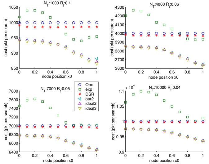
**Figure 5: Cost of different schemes for nodes at different locations in small-scale networks. The X-axis indicates the location of the investigated nodes. The Y-axis indicates the cost of different schemes. Different network sizes of 1000, 4000, 7000 and 10000 nodes are simulated. The tested schemes are: the once-for-all scheme, the DSR scheme, the expansion ring scheme, our two-tier scheme, the ideal two-tier scheme and the ideal three-tier scheme.**
