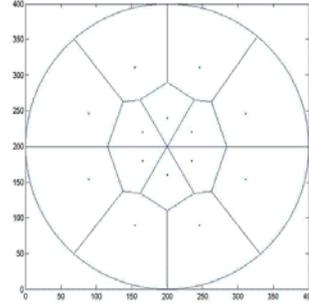
Fig. 1) The Voronoi tessellation of a network where cluster heads are arranged circularly around the base station.
