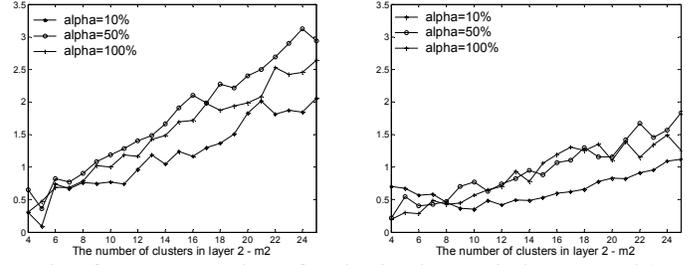
Ratio of average number of nodes in clusters in layer 1 and 2 in UCS, for a network with static clusters.
