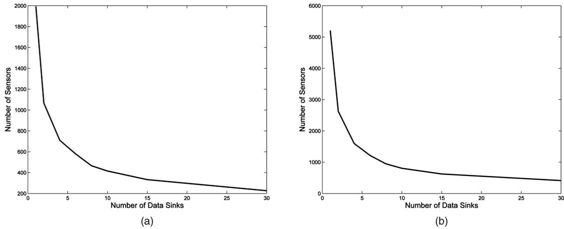
Fig. 9. Number of sensors required to meet the target scenario lifetime (a) when using transmission power control and (b) when not using transmission power control for the multiple-data-sink deployment strategy.
