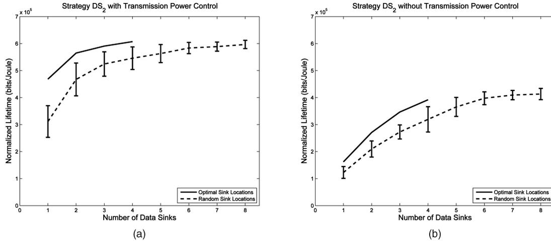
Fig. 5. Normalized lifetime versus number of data sinks deployed for the sample scenario (a) with transmission power control and (b) without transmission power control. Increasing the number of sink locations improves the lifetime until a certain threshold is met and the hot-spot problem has been effectively solved.
