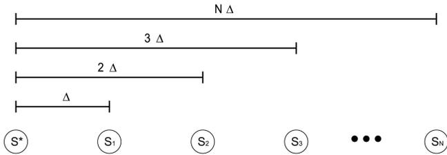
Fig. 1. A one-dimensional regularly spaced network topology. Nodes are equally spaced in this scenario.
