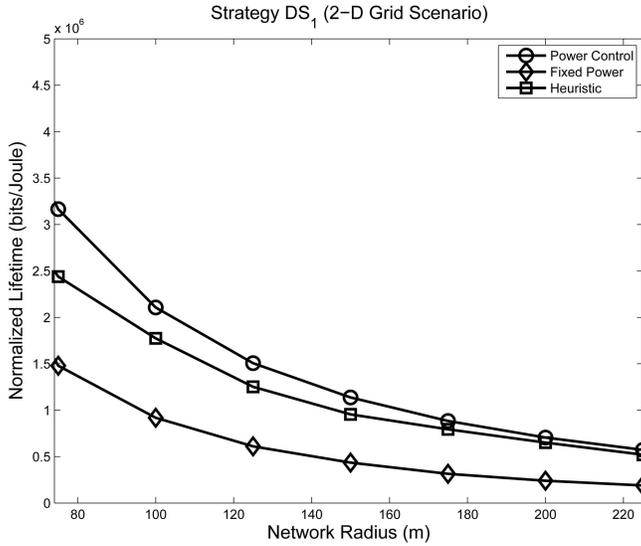
Fig. 3. Network lifetime as a function of the network radius for the optimal power control scheme, the fixed transmission power scheme, and the heuristic power control scheme in a 2D scenario.
