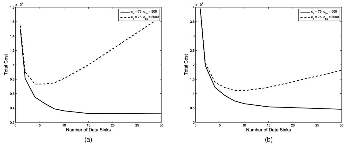
Fig. 10. Total cost of deployment for the target scenario (a) when using transmission power control and (b) when not using transmission power control for the multiple-data-sink deployment strategy.
