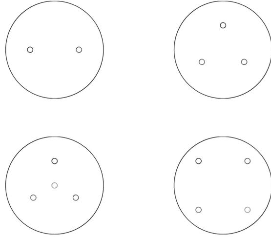
Fig. 4. Sink locations can be presumed to be in a symmetric pattern. The pattern for less than five sinks can thus be determined as shown.
