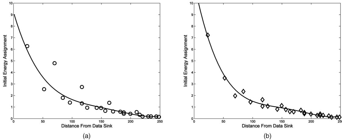
Fig. 8. Energy distribution map for the sample scenario (a) with transmission power control and (b) without transmission power control. Nodes closest to the base station should be assigned the most energy. The assignment can be approximated using a polynomial function.
