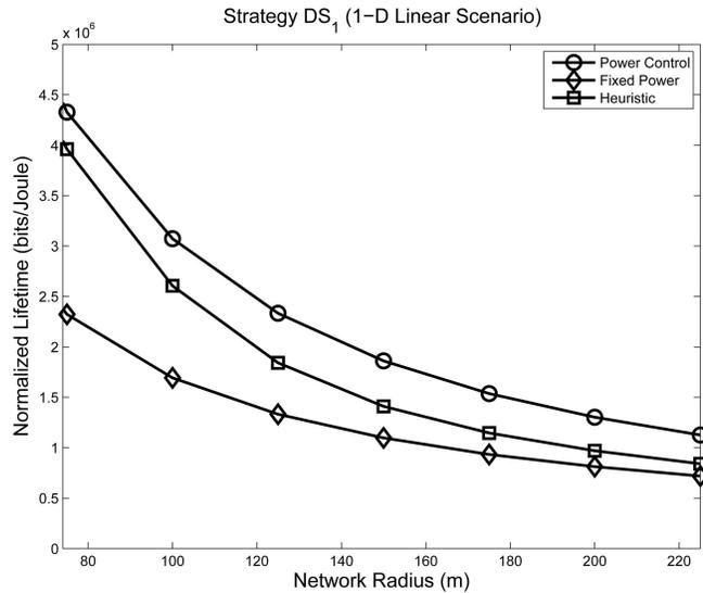
Fig. 2. Network lifetime as a function of the network radius for the optimal power control scheme, the fixed transmission power scheme, and the heuristic power control scheme in a one-dimensional scenario.
