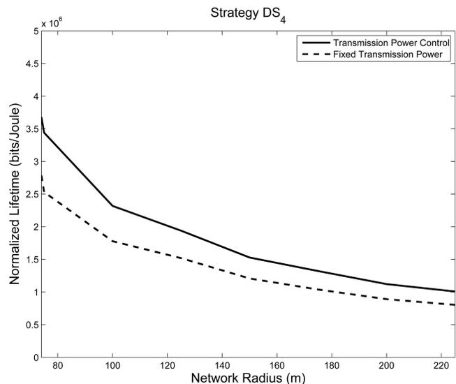
Fig. 7. Normalized lifetime as the network radius varies for the nonuniform energy assignment strategy.
