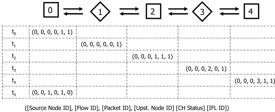
Fig. 5. Illustration of IFL and IS contents. Squares and diamonds represent CHs and ordinary nodes, respectively. Node-0 is the source node. The entries below the nodes represent the contents of ([Source Node ID] [Flow ID] [Packet ID] [Upstream Node ID] [(CH Status)] [IFL ID]) fields of their IS packets ( $t_{iS}$  represent time instants).
