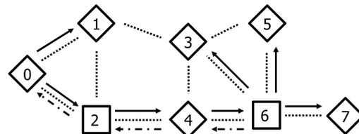
Fig. 6. Illustration of IFL and PRN. Squares and diamonds represent CHs and ordinary nodes, respectively. Node-0 is the source node. Dotted lines represent the links between the nodes. Solid and dash-dotted lines represent the data and IS flows, respectively.
