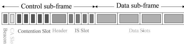
Fig. 2. MH-TRACE frame structure.
