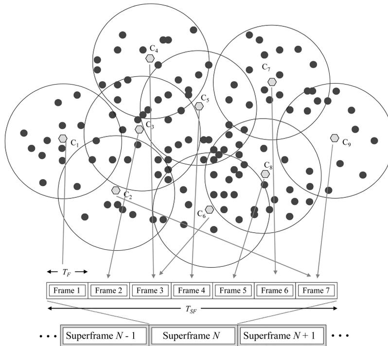
Fig. 1. A snapshot of MH-TRACE clustering and medium access for a portion of an actual distribution of mobile nodes. Nodes  $C_1 - C_9$  are CHs.
