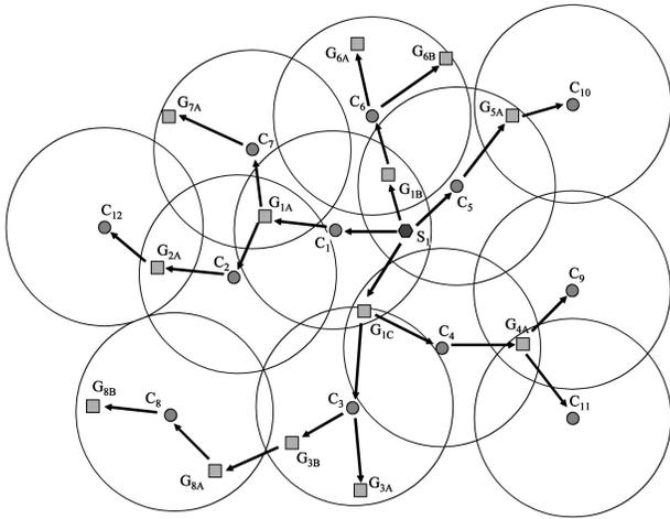
Fig. 3. Illustration of NB-TRACE broadcasting. The hexagon represents the source node, disks are clusterheads, the large circles centered at the disks represents the transmit range of the clusterheads, squares are gateways, and the arrows represent the data transmissions.
