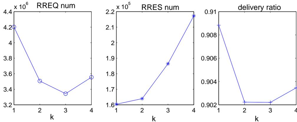
Figure 4.8: Performance of DSR-LC with  $p_t$  fixed at 0.4. The X-axis indicates the local searching radius  $k$ , ranging from 1 to 4. The optimal point is at  $k = 3$  for the number of RREQ with almost no effect on other metrics.
