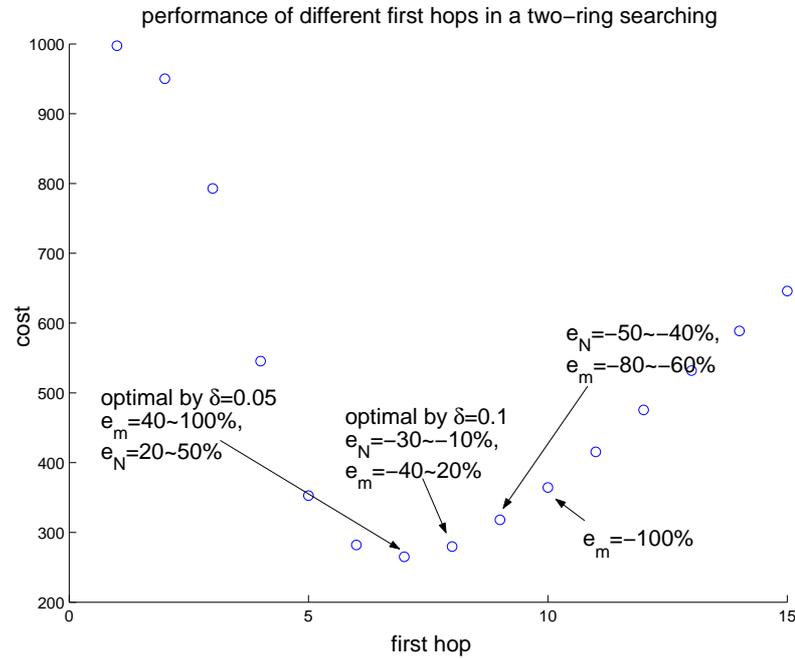
Figure 3.8: The cost for all the possible first hops using a two-ring searching in small-scale networks. The x-axis indicates the first hop limit. Erroneous network parameter estimations result in erroneous hop limit choice. Substantial cost saving can still be achieved using erroneous parameters.
