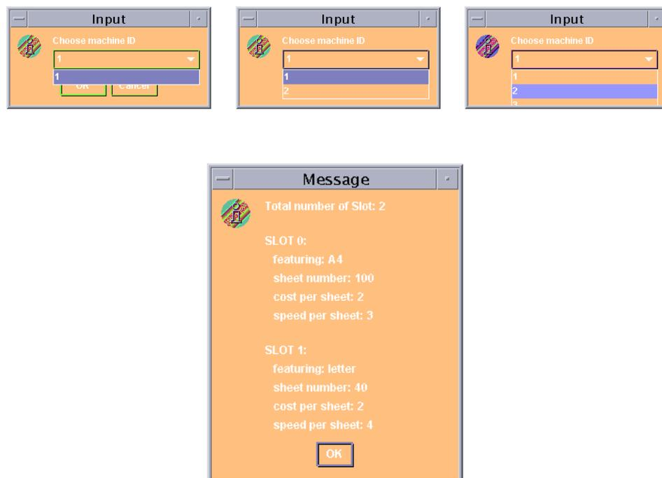
Figure 7.6: Status service: the information about the printers' status grows at the MASTER as new nodes join the network. This is implemented by the MASTER periodically polling the peers. The peers' printer status is stored in the MASTER for use in resource allocation.
