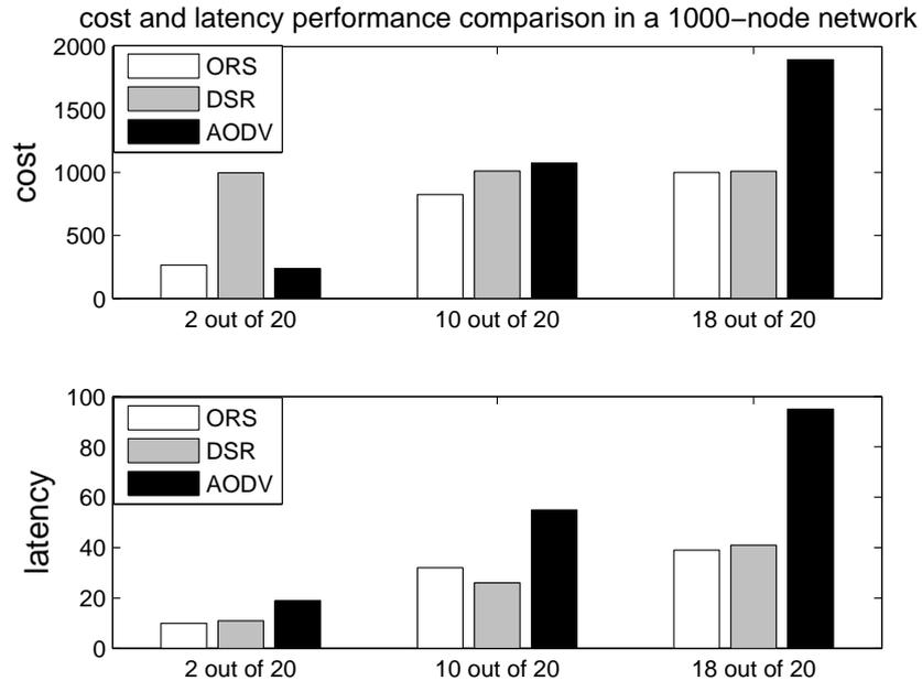
Figure 3.7: Searching cost and latency comparison in small-scale networks for self-location unaware nodes. RS performs consistently close to optimal in terms of both cost and latency for all searching tasks.
