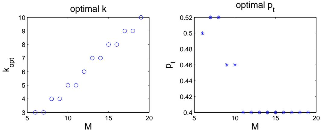
Figure 4.5: The optimal parameters  $k$  and  $p_t$ . The optimal  $k$  value is consistently around  $\frac{M}{2}$ . The optimal  $p_t$  is around 0.4 to 0.5, depending on the the maximum hop radius  $M$ .
