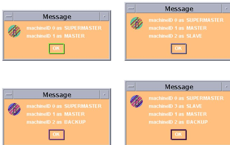
Figure 7.5: Presence service: nodes 1, 2 and 3 join in the network and determine their roles automatically. These figures show the results of node 1, the MASTER node, executing the presence service at different times.
