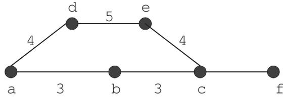
Figure 5.3: An example showing how the delay rules can help set up both the primary and the auxiliary routes.
