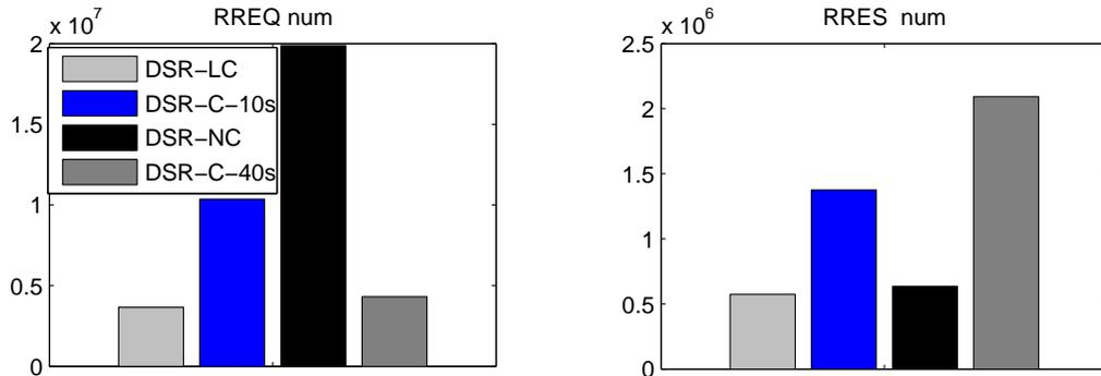
Figure 4.12: Routing overhead comparisons under a high event rate of 0.5 events/sec and a low maximum node speed of 1m/s. This figure shows the performance of different schemes in an abundant caching condition.
