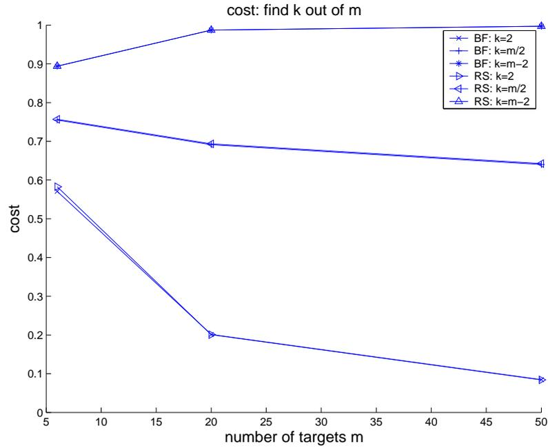
Figure 3.4: The optimal expected cost for  $k$ -out-of- $m$  discovery by different algorithms. The x-axis indicates the targets available in the searching area. The y-axis indicates the expected cost. 2,  $\frac{m}{2}$ ,  $m - 2$  targets are to be searched for each algorithm.
