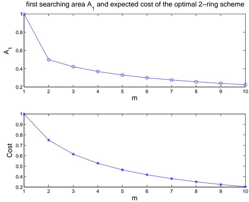
Figure 3.2: 1-out-of- $m$ , the optimal two-ring scheme. The optimal first searching area  $A_1$  (top graph) and the corresponding cost  $C$  (bottom graph). The values vary according to the number  $m$  of existing targets. The more targets available, the smaller the first searching area and the less expected cost are.
