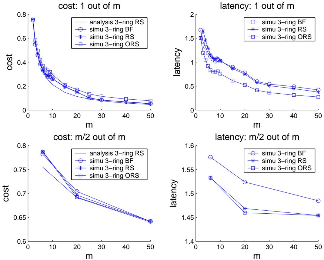
Figure 3.5: The average cost and latency performance for each algorithm for geographical scenarios. The x-axis indicates the targets available in the searching area. The top row shows the results of 1-out-of- $m$  discovery, and the bottom row shows the results of  $\frac{m}{2}$ -out-of- $m$  discovery.
