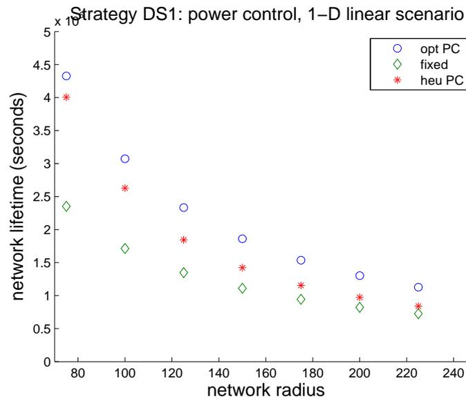
Figure 6.2: Network lifetime as a function of network radius for the optimal power control scheme, the fixed transmission power scheme and the heuristic power control scheme in a one-dimensional scenario. X-axis indicates network radius, and Y-axis indicates the maximum achievable network lifetime. “Opt PC” represents the optimal power control scheme, “fixed” represents the fixed transmission power scheme, and “heu PC” represents the heuristic power control scheme.
