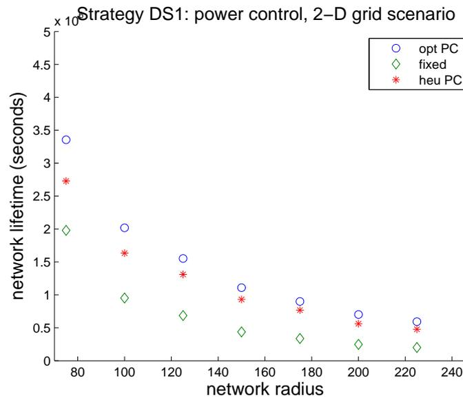
Figure 6.5: Network lifetime as a function of network radius for the optimal power control scheme, the fixed transmission power scheme and the heuristic power control scheme in a two-dimensional scenario. X-axis indicates network radius, and Y-axis indicates the maximum achievable network lifetime. “Opt PC” represents the optimal power control scheme, “fixed” represents the fixed transmission power scheme, and “heu PC” represents the heuristic power control scheme.
