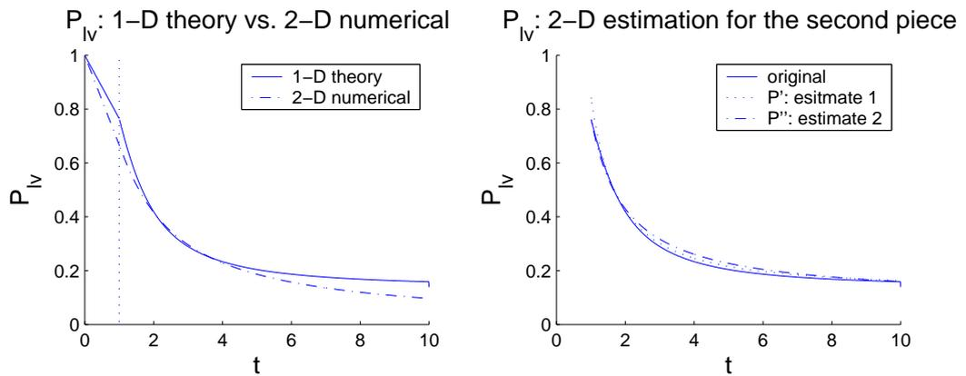
Figure 4.4: The  $P_{lv}(t)$  in 1-D and 2-D cases. On the left figure, the theoretical results of  $P_{lv}(t)$  in a 1-D case and the numerical results in a 2-D case are shown. They both have a two piecewise tendency. On the right figure, two estimations for the 2-D numerical results are shown.
