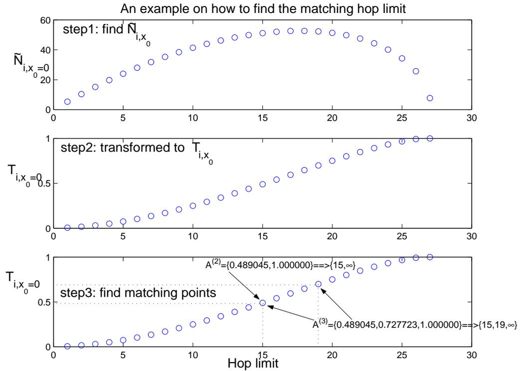
Figure 3.6: An example on how to transform calculated areas into hop limits. First,  $N_{i,x_0}$  is estimated. Second, normalized  $T_{i,x_0}$  is determined. Finally, hop limits can be found by matching the areas with  $T_{i,x_0}$ .
