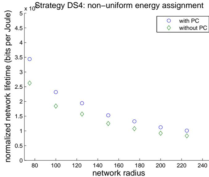
Figure 6.9: Normalized lifetime for different network radius. Power control is no longer important once energy can be freely assigned.
