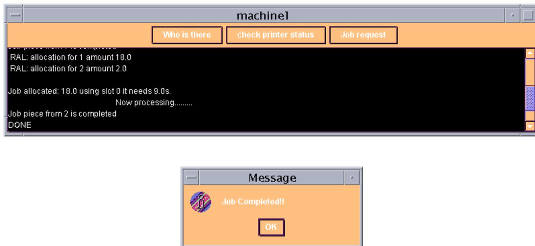
Figure 7.11: Job dispatch service: after a user accepts a price quote, the MASTER dispatches pre-calculated job pieces to pre-assigned machines. The MASTER sends a job completion notification to the user at the requesting terminal once all job pieces are completed.
