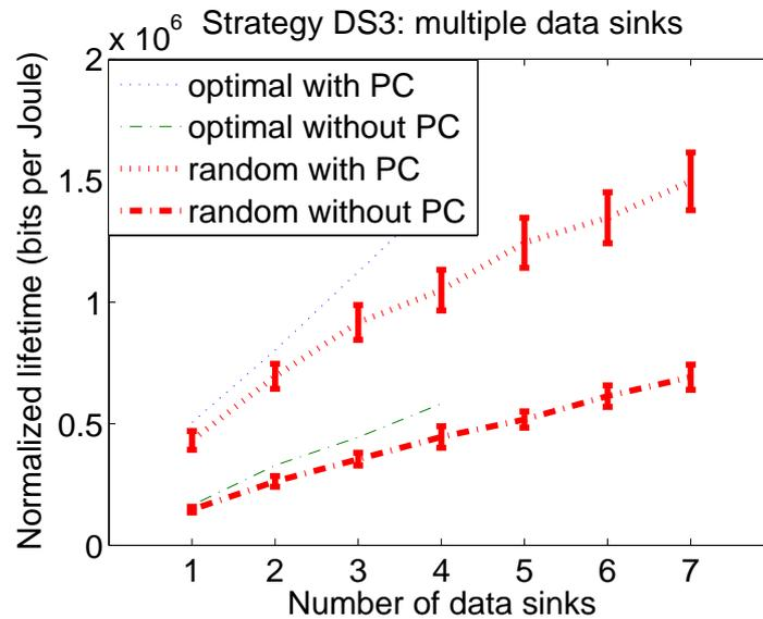
Figure 6.8: Normalized lifetime vs. number of cluster heads deployed. Large gains in network lifetime can be achieved when even a few extra cluster heads are deployed, especially when their locations are optimized. Random sink locations can provide lifetime improvement, but it is not as large as that obtained using the optimal sink locations. When power control is unavailable, the gap between random sink locations and optimal sink locations is greatly reduced.
