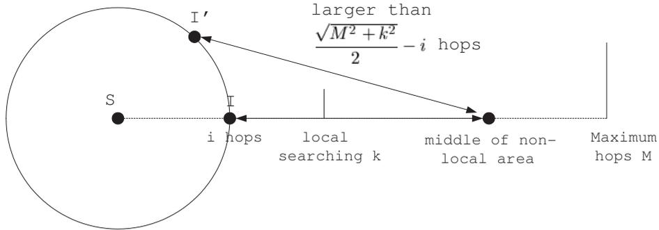
Figure 4.2: Local searching example. The shortest distance from the intermediate node that is  $i$  hops away from the source node to the middle of the non-local area is  $\frac{\sqrt{M^2+k^2}}{2} - i$ .  $k$  is the local searching radius and  $M$  is the maximum hop of the network.
