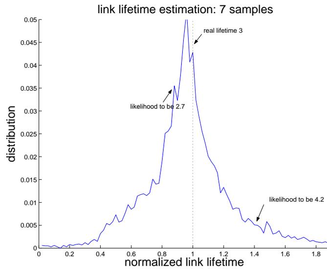
Figure 5.6: Link lifetime estimation error pattern. The X-axis indicates the normalized link lifetime estimation. The Y-axis indicates the probability distribution of lifetime estimation. For example, when the real lifetime is 3, the likelihood of estimation as 2.7 is 7 times that of estimation as 4.2.
