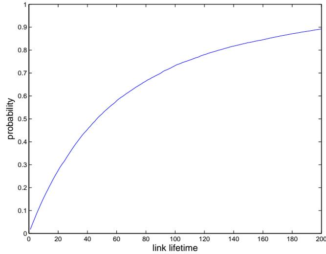
Figure 5.1: Link lifetime distribution in the Gauss-Markov scenario.
