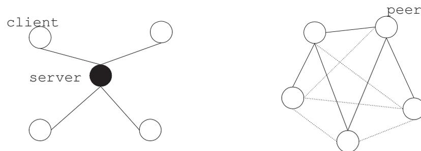
Figure 7.1: A high-level view of the client/server model and the P2P model.
