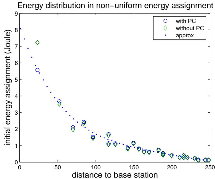
Figure 6.10: Energy distribution map for the sample scenario. Nodes far from the base station should be assigned more energy. The assignment can be approximated using a polynomial function shown by the dotted line.
