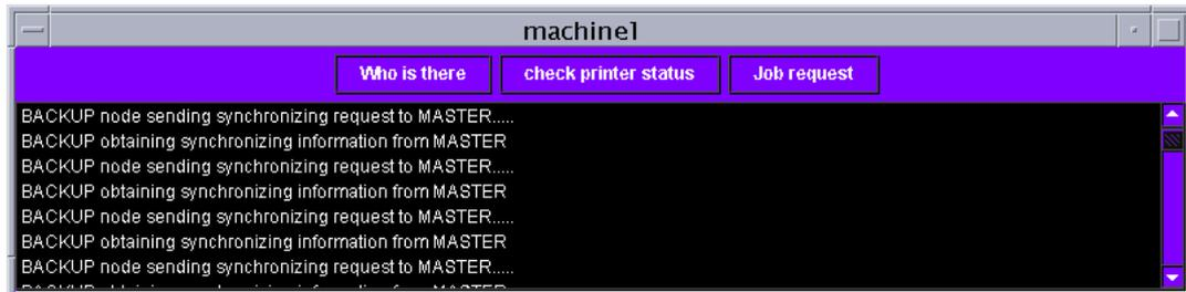
Figure 7.7: Synchronization service: a BACKUP synchronizes with a MASTER periodically.
