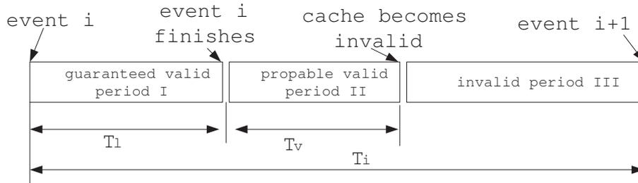
Figure 4.1: Time periods for a node's route caching between two events towards the same destination. During the guaranteed valid period I, the node has traffic and maintains the cache. In the probable valid period II, the node has stopped sending traffic to the destination and therefore has only a probable valid route cache. In the invalid period III, the route caching valid probability is so low that this route cache may be discarded.
