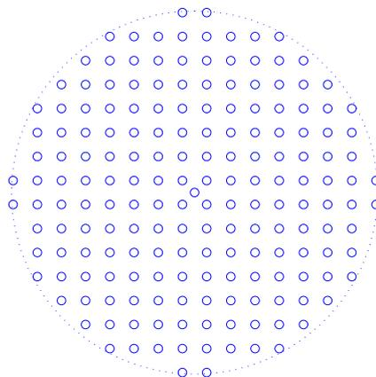
Figure 6.3: The 2-D circular grid topology. 180 nodes are placed within the circle area in this plot.
