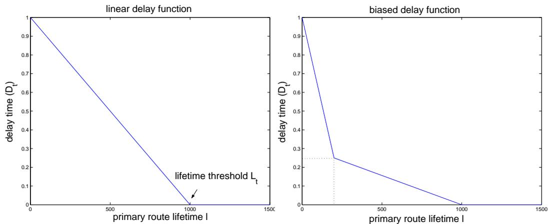
Figure 5.5: The delay function  $f(l; D_1)$ . On the left is a simple linear function. On the right is a biased linear function to concentrate on the first 200 seconds.
