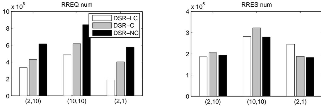
Figure 4.11: Routing overhead comparisons under a low event rate of 0.05 events/sec. The X-axis indicates different scenarios tested, from left to right stands for (event life, node speed) pairs of (2s, 10m/s), (10s,10m/s), (2s,1m/s). This figure shows the effects of event lifetime and the node speed on routing overhead in a moderate caching condition.
