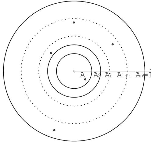
Figure 3.1: The simplified model of target discovery. The searching areas are concentric circles. Both the target nodes (black dots) and non-target nodes (not shown) are uniformly distributed in the searching area.
