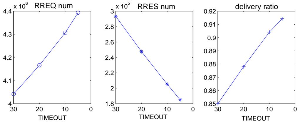
Figure 4.10: Performance of DSR-C with one-hop neighbor searching. The X-axis indicates the timeout value, ranging from 30 seconds to 5 seconds. The tradeoff is also between the RREQ number and the delivery ratio. Just like Fig. 4.9, the increase of TIMEOUT causes both metrics to decrease. A good balance point is at TIMEOUT=10 seconds.
