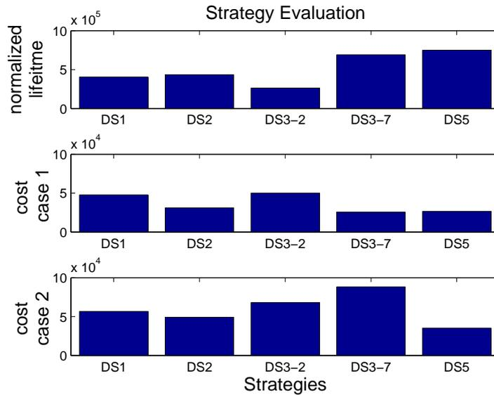
Figure 6.11: Evaluation of the following sensor network deployment strategies: power control ( $DS_1$ ), mobile base station ( $DS_2$ ), multiple base stations ( $DS_{3-2}$ ,  $DS_{3-7}$ ) and non-uniform relay assignment  $DS_5$ . The first row is the normalized lifetime. The second row is the deployment cost for the target scenario for cost case 1, and the third row is the deployment cost for the target scenario for cost case 2.
