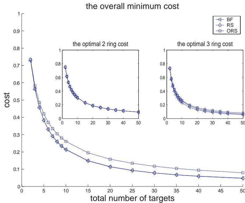
Figure 3.3: The optimal expected cost of finding one target for each algorithm and the optimal 2-ring and 3-ring cost for each algorithm. The x-axis indicates the targets available in the searching area. The y-axis indicates the expected cost. Although the number of rings  $n$  to achieve the overall optimal cost is usually larger than 3, the optimal 3-ring scheme already performs very close to the real optimal.
