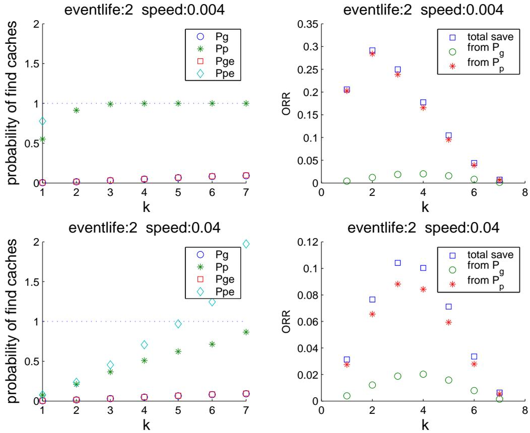
Figure 4.6: The scenarios for event lifetime as low as 2 seconds. The maximum node speed is either 0.004 (upper part) or 0.04 (lower part). The X-axis indicates the local searching radius  $k$  and the Y-axis indicates  $P_g$  and  $P_p$  and their estimations  $P_{ge}$  and  $P_{pe}$  in left figures and  $ORR$  in right figures. The estimation of  $P_p$  go beyond 1 at hop 2 and cannot be seen in the upper left plot.
