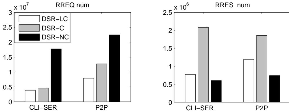
Figure 4.13: Routing overhead comparisons for peer-to-peer and client-server traffic models.
