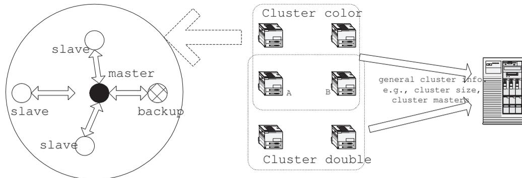
Figure 7.2: A hybrid clustering scheme for the smart document system.
