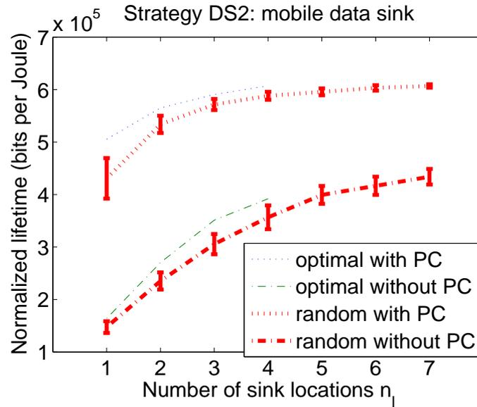
Figure 6.7: Normalized lifetime vs. number of data sinks deployed for the sample scenario. Increasing the number of sink locations improves lifetime until a certain threshold is met and the hot spot problem has been effectively solved.
