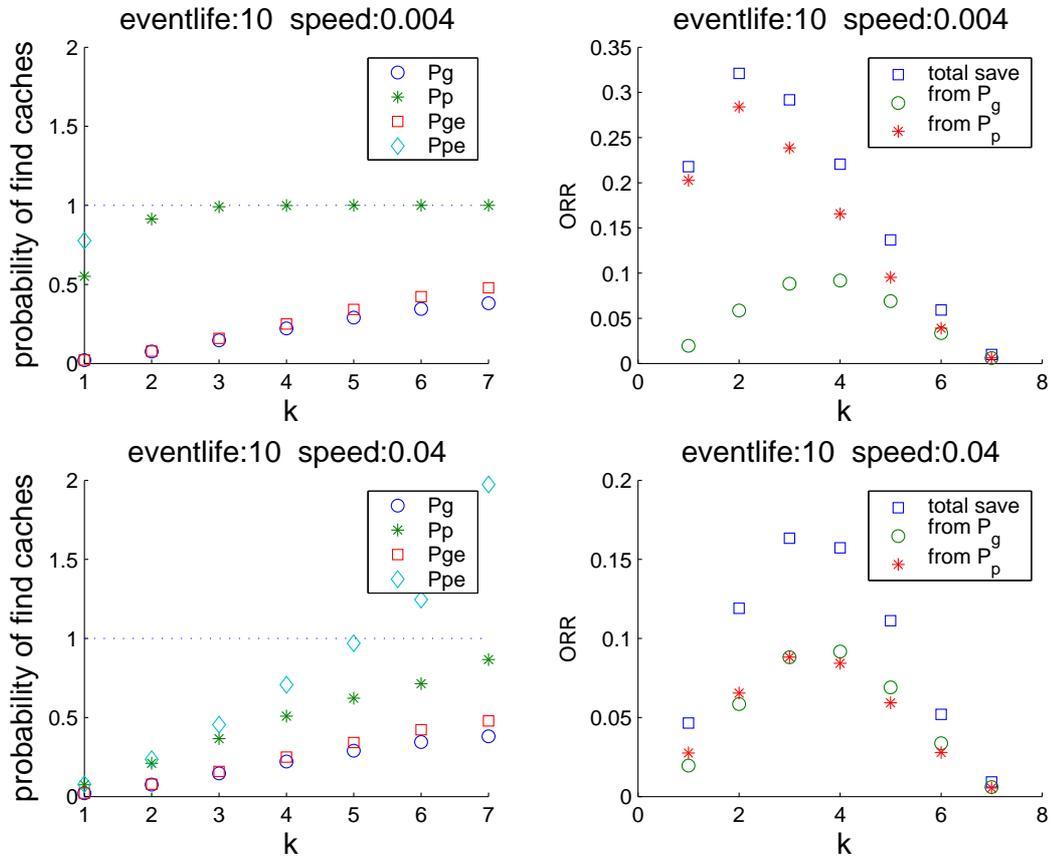
Figure 4.7: The scenarios for event lifetime as high as 10 seconds. The maximum node speed is either 0.004m/s (upper part) or 0.04m/s (lower part). The X-axis indicates the local searching radius  $k$  and the Y-axis indicates  $P_g$  and  $P_p$  and their estimations  $P_{ge}$  and  $P_{pe}$  in left figures and  $ORR$  in right figures. The estimation of  $P_p$  go beyond 1 at hop 2 and cannot be seen in the upper left plot.
