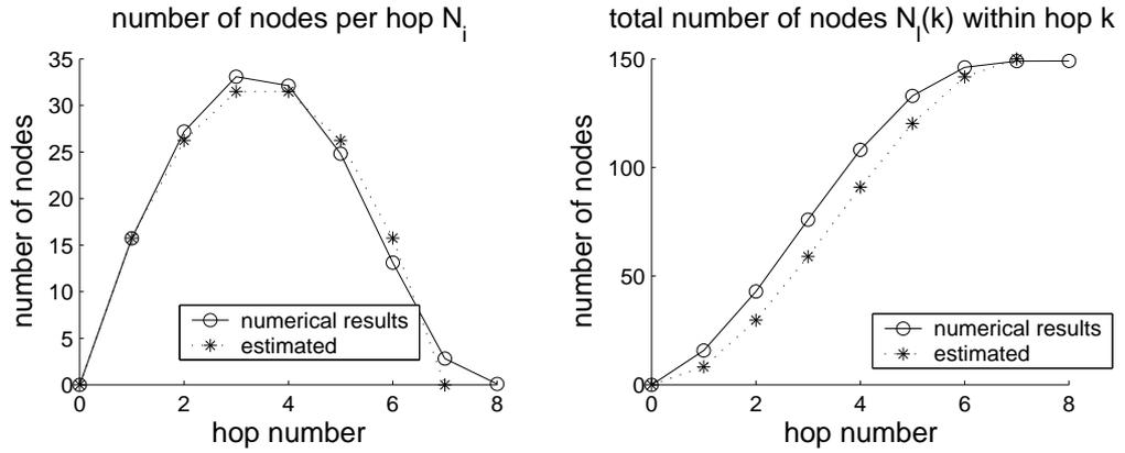
Figure 4.3: The number of nodes at each hop  $N_i$  (left) and the number of nodes within  $k$  hops (right). Both the experimental results and their estimates are shown.
