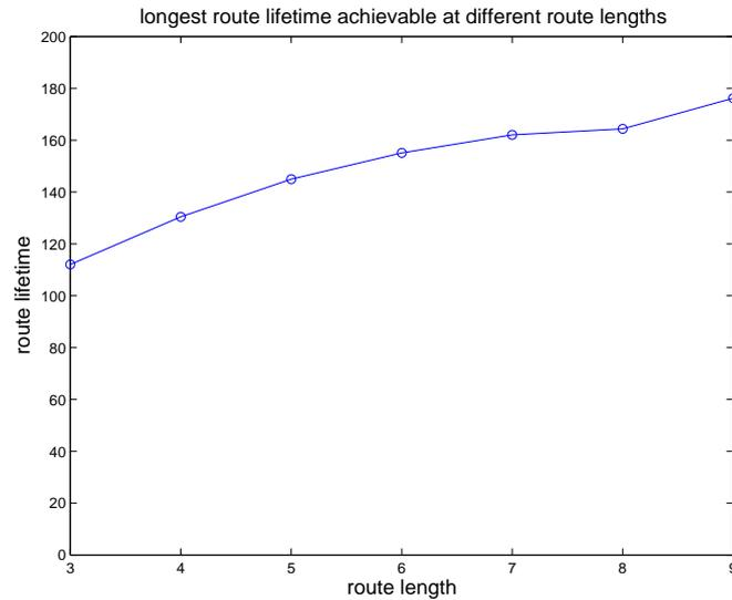
Figure 5.2: The longest lifetime achievable for routes of different route lengths. A linear tendency is shown.
