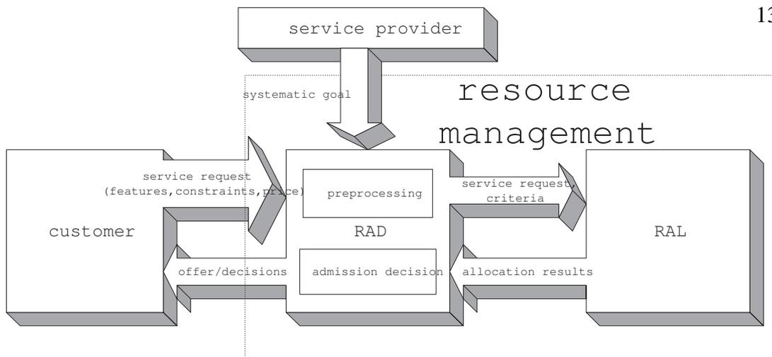
Figure 7.3: The resource management module, its components RAL and RAD and their relation with the service provider and the customer.
