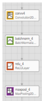
Fig. 2. A single CNN block design includes a convolutional layer, batch normalization layer, ReLU and maxpool. [2].
