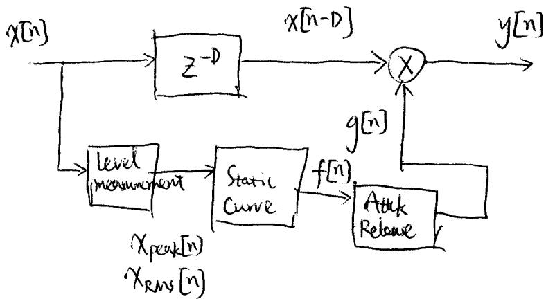
Spectrum of  $y[n]$  is convolution of spectrum of  $x[n]$  and spectrum of  $g[n]$ .
