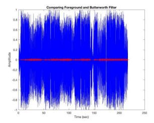
**Fig. 4**. Implementation of the Butterworth filter on the isolated vocal track. The isolated vocal track is shown in blue, and the low-frequency removed audio is shown in red. Cut-off frequency is at 100 hertz.
