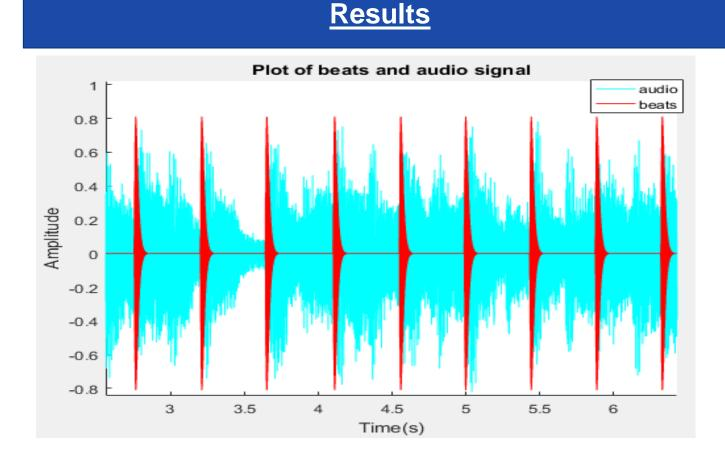
Plot of the beats detected against the audio signal specified. Note beats are detected at the beginning of the onsets in the signal.
