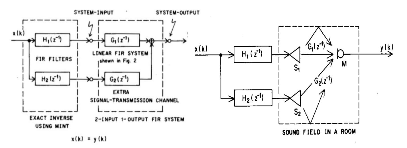
We form the following Toeplitz matrix G containing the IRs G1 and G2. The exact inverses H1 and H2 can then be computed using inv(G) and the Delta Matrix D.
