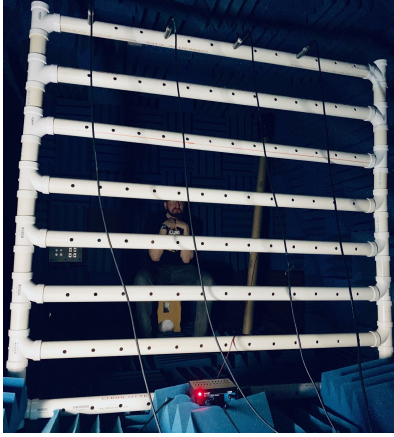
Figure 2: Recording Apparatus in the Anechoic Chamber
