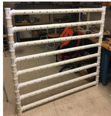
Figure 1: PVC Base of WFS Driver Array
