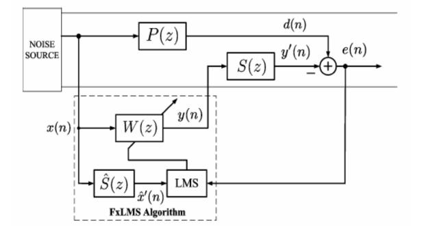
applications, real-time the For is consisted of secondary path amplifier, DAC, reconstruction filter and the loudspeaker, etc. And will not always be stationary. Therefore, updating secondary path is required and critical for some ANC systems.
