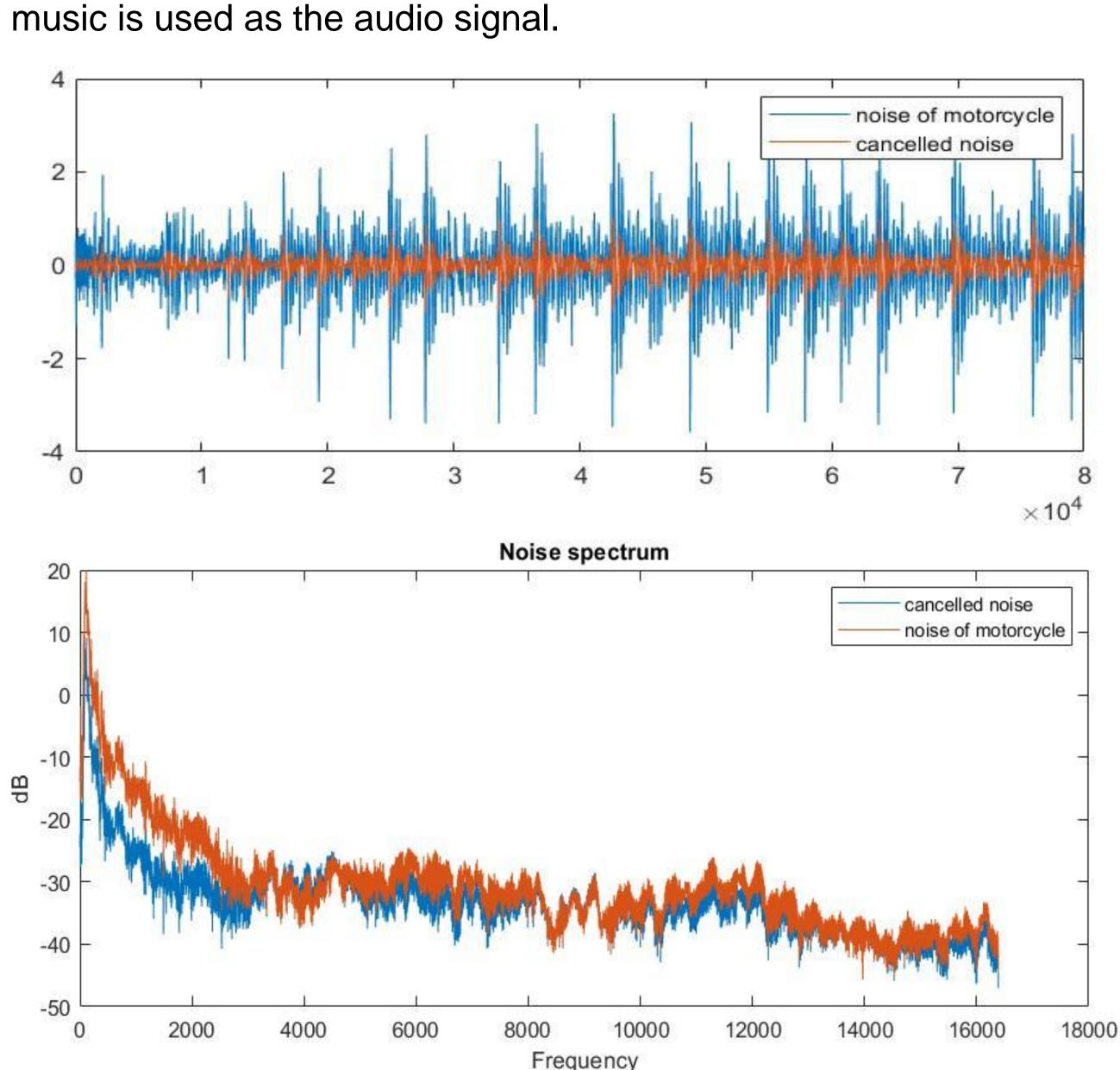
• The audio integrated noise control system can effectively cancel the low frequency noise signal below 1000Hz while playing the desired audio signal.
