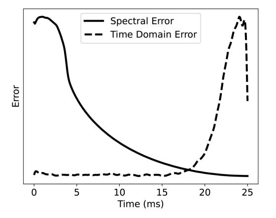
To use the middle most-sensitive region, output should be windowed and hopped at 50%.
