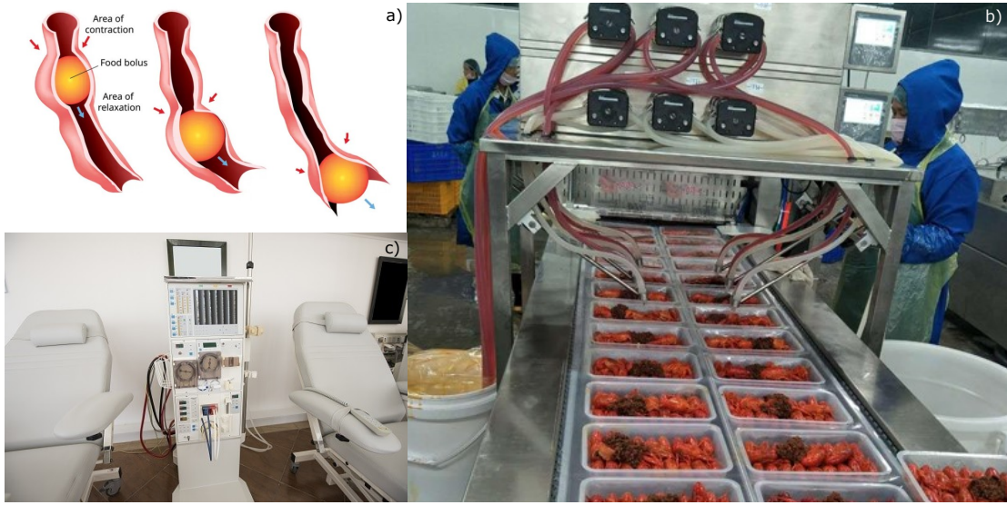
Figure 2.6: Shown are examples of systems where one can find peristaltic pumping: a) Pumping in the stomach [4, 5]. b) Industrial applications on food processing [6]. c) Applications in medical pumps [7].
