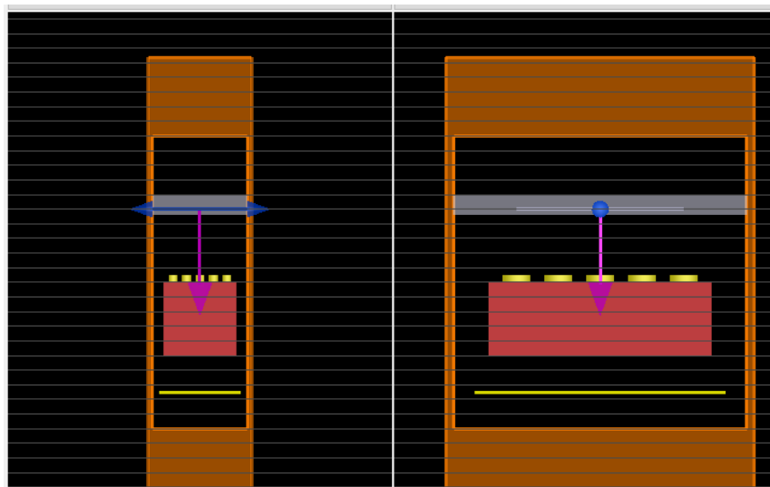
Figure 04: Array of 50nm tall gold pillars nested on top of a silicon substrate using Lumerical FDTD Solutions. This was too complex of a simulation to run, but the computers in the Hopkins Center will be able to run it.
